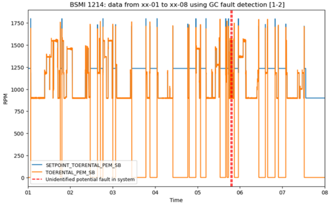
FIGURE 5.16: Results of the second fault detection test for application 1 showing only unidentified faults
