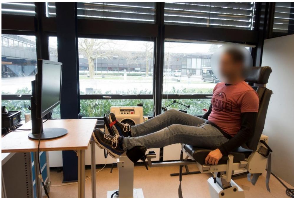
Figure 3: Setup showing the subject seated in the chair in front of the dynamometer with the right foot fixed on the footplate and the screen in front of the subject.
