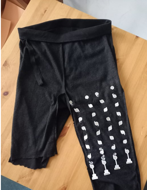
Fig. 4: The wearable electrode-embedded garment. Only the backside is shown, but electrodes are also present at the front. The leggings are cut short to increase subject comfort.
