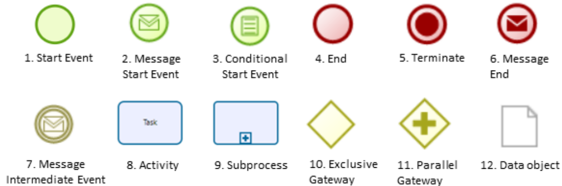
Figure 2.1: Symbols used in the business process model (Bizagi, One Platform; Every Process. User Guide Modeler, nd)
