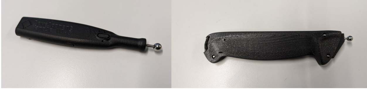
Fig. 6. The Inverse3 handle (left) and 3D printed knife (right) next to eachother
