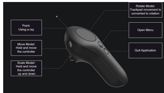
Figure 3.10: The magic leap controller with controls for the AR environment.
