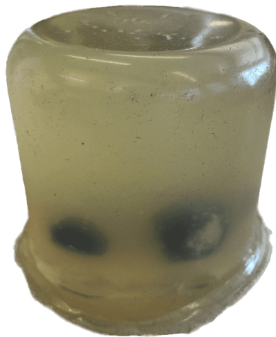
Figure 3.5: The made phantom from PVC. The blue parts are the tumors.
