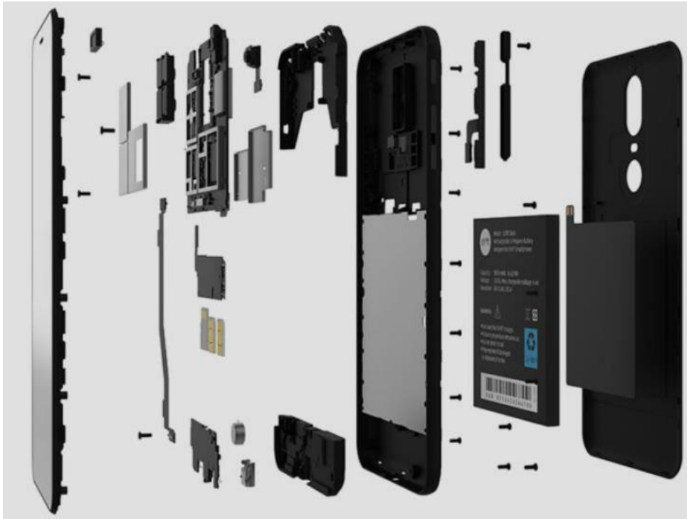
Figure 3 Modular smartphone design of Shiftphone(2023), https://www.shift.eco/en/circular-economy-and-the-13-shiftcycles-part-3-redesign/
