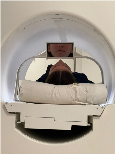
Fig. 7: Subject lying inside MRI tunnel bore with the mirror attached to the head coil. The nose/mouth region of interest can be seen in the mirror. The subject would be wearing a mask and the thermal data would be picked up by the camera.
