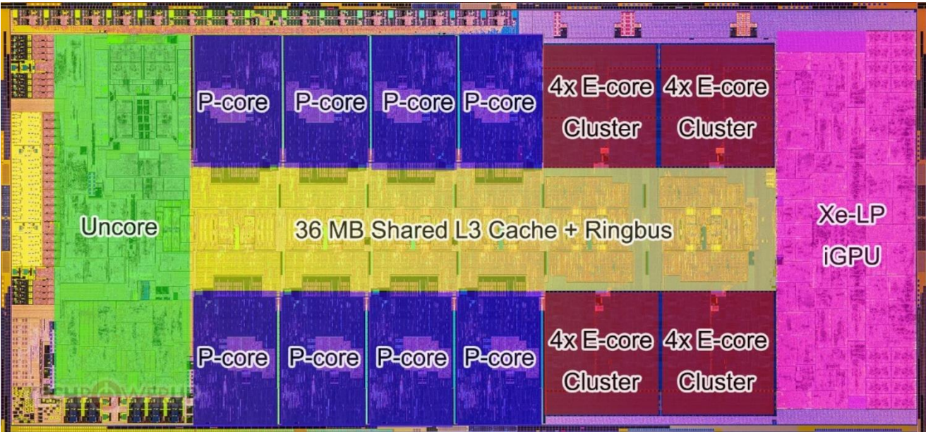
Figure 29: Intel core Raptor Lake CPU microarchitecture (Intel Core i5-13600K, 2022)
