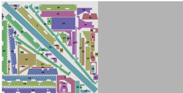
FIGURE 8: The cutting order of the second example, resulting from Nest&Cut, after running the nest for 5 minutes.
