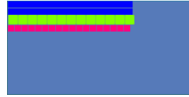
(B) Manual adjusted solution maximizing the remnant sheet by employing an L-shaped cut.
