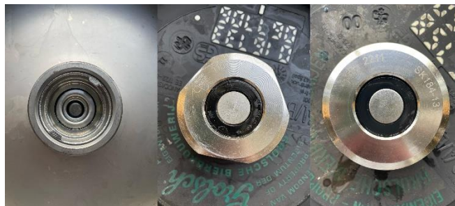
Figure 2.7: S-fitting; G-fitting; A-fitting
