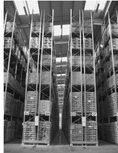
Fig. 5: Narrow aisle racking
