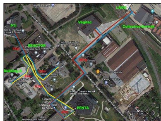
Figure 11 - Current Heat Grid Kortrijk Weide (lines)
