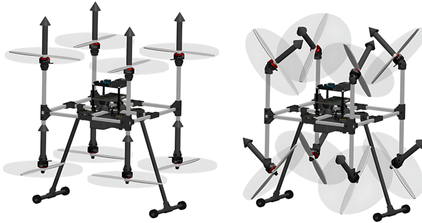
Figure 1.1: The OmniMorph platform. Left: OmniMorph in its most energy-efficient mode with all rotors pointing upwards. Right: OmniMorph in its omnidirectional mode, allowing it to hold its position in any orientation. Source: Aboudorra et al. (2024)
