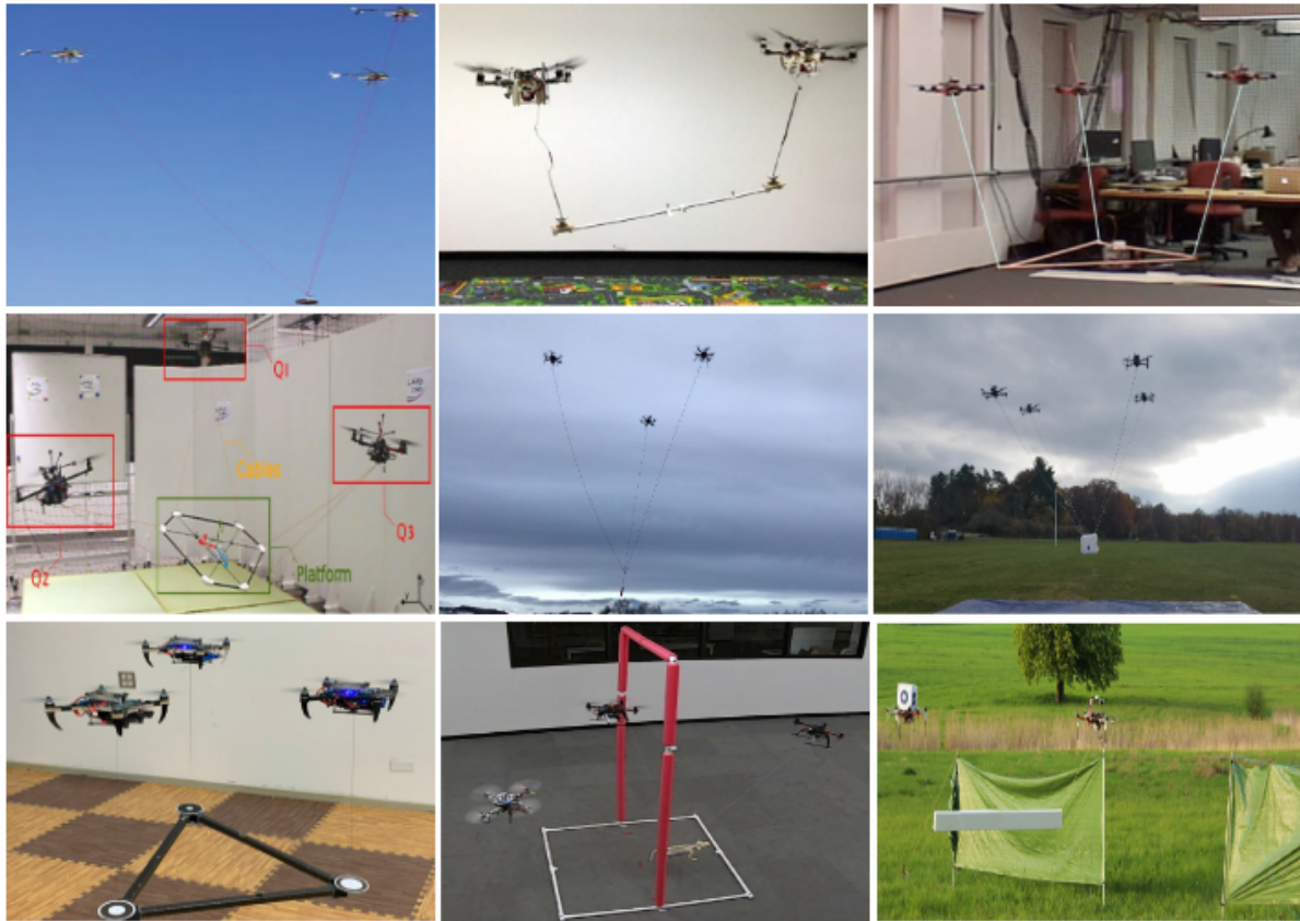
Figure 1.5: Different works of co-operative aerial transportation objects using taut cables, shown as a survey in [6]
