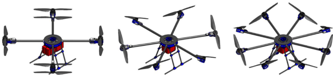
Figure 1.3: Different Multi-rotor aerial platforms with rotor tilt mechanisms for full actuation as shown in [29]
