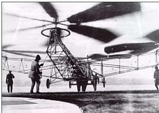
(c) The real working Bothezat quadrotor for the US army around 1924 [24]
