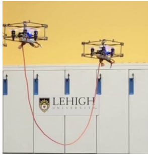
(a) Manipulating hook shaped objects based on catenary model of cable with 2 quadrotors [13]
