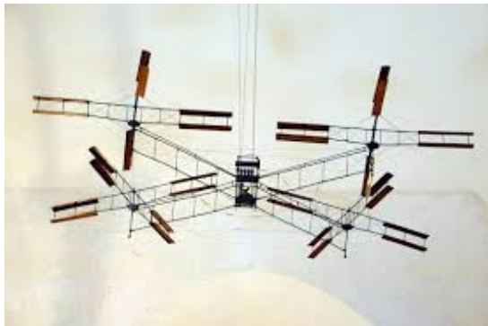
(a) A miniature version of the first quadrotor (gyroplane 1) in paris museum, original version built by Jacques in 1907 [23]
