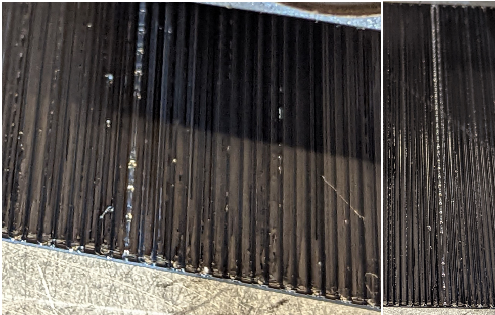
(b) Inconsistent print in internal layer.
