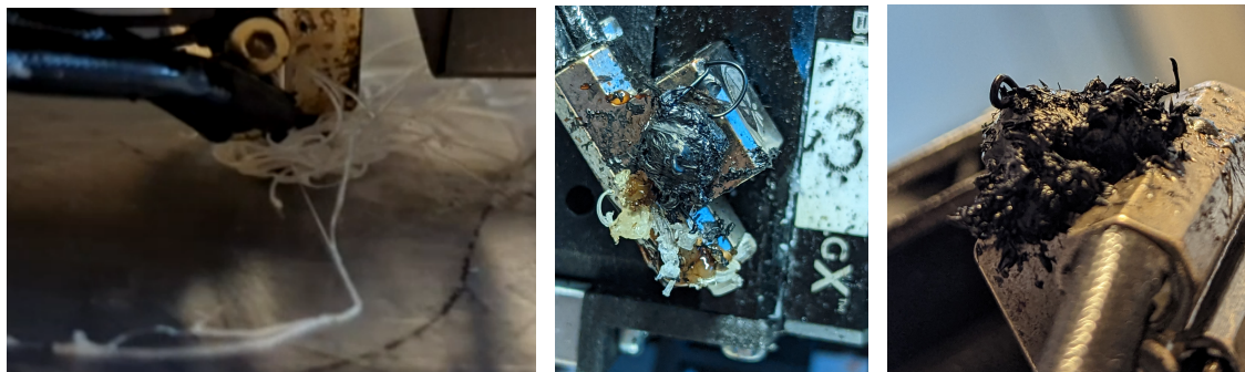
(a) Nozzle clog experienced while printing the support material, BVOH.
