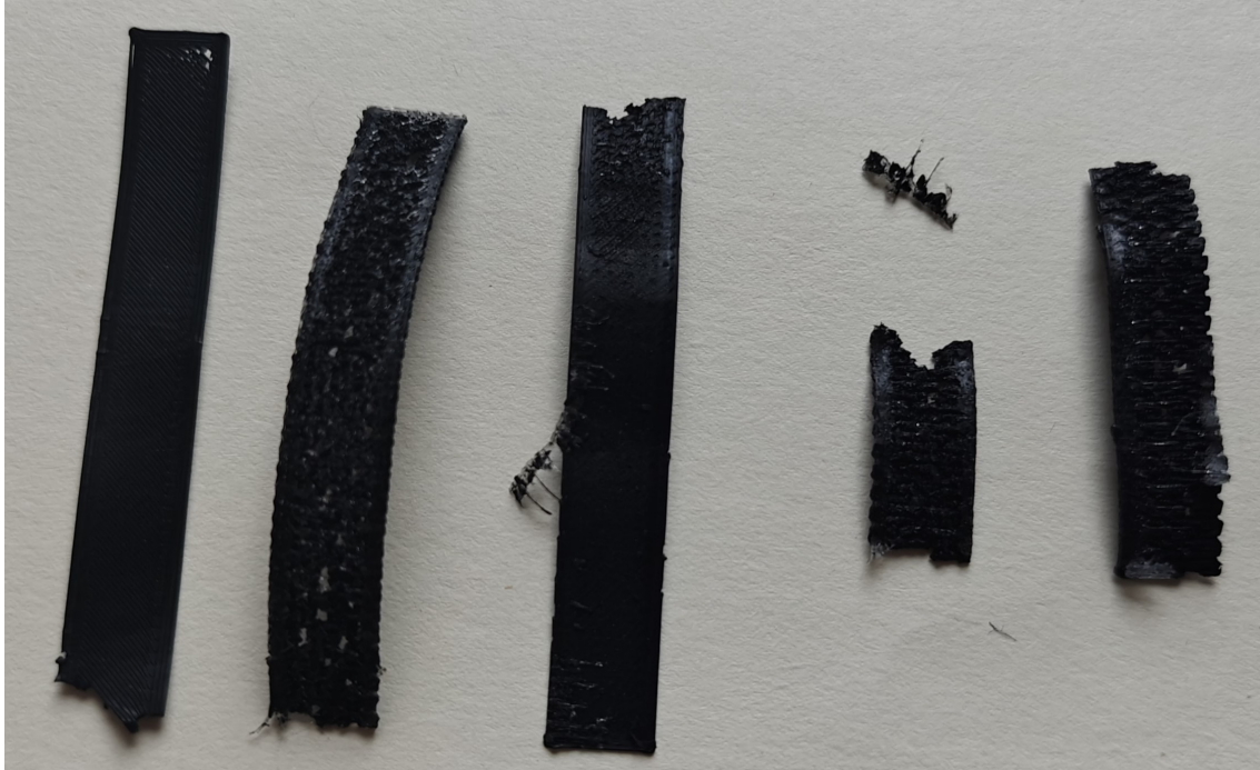
Figure 6.17: Dismantled sensor print with misprinted dielectric.
