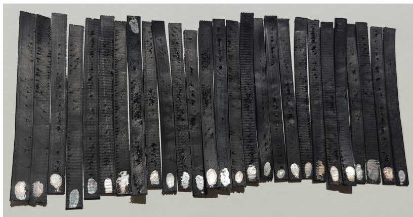
(d) Sensors with holes on the top layer, because of under-extrusion [112].
