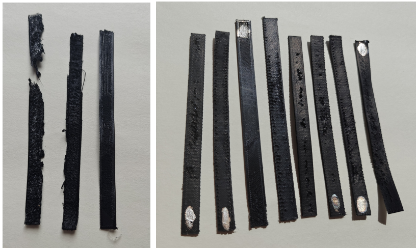
(a) Sensor misprint before top layer is printed. (b) Various types of issues on the printed sensors.
