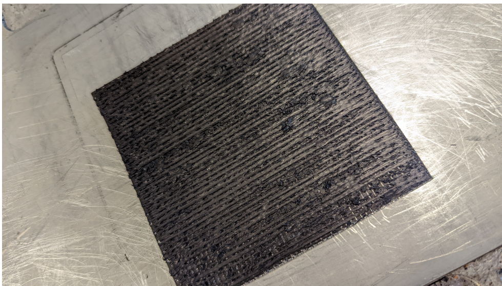
(c) Zits seen on the top layer because of misprints in the internal layers of the sensor.
