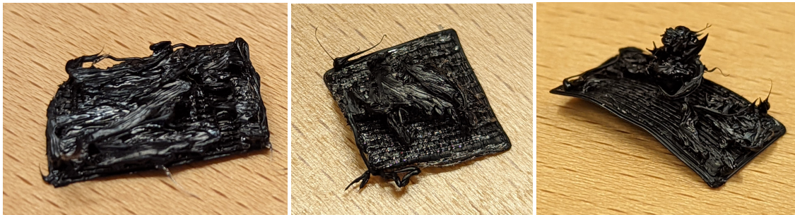
Figure 4.4: Printed output of test samples with various print temperatures and print speeds.
