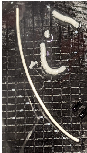
Figure 4.2: Dissolution of BVOH(left) versus PLA(right)
