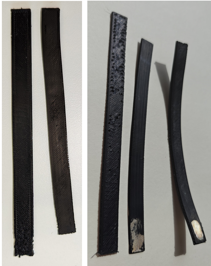
Figure 6.23: Sensor prints before and after (shrunken) baking.
