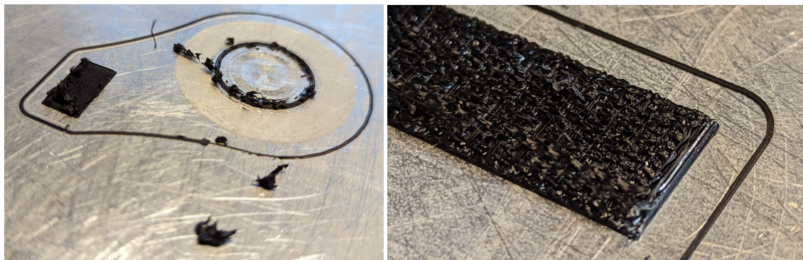
(a) Issues in printing the top layer.
