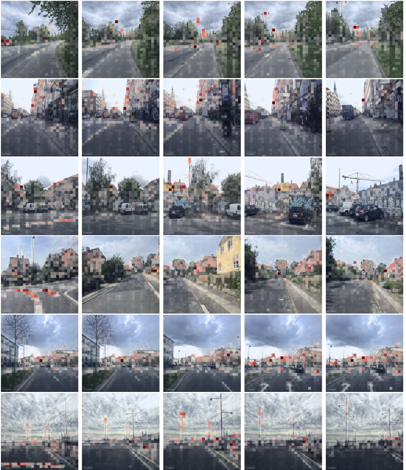
FIGURE 7: Visualization of the attention map for the last layer of the encoder using the method DINOv2 + SeqVLAD, for image sizes 392x392. The attentions for the 12 attention heads of the CLS token are averaged and the attention map is overlaid on the original image using a red hue. This figure shows that the model focuses on static visual features such as road markings and buildings and ignores movable objects like cars.
