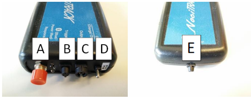
Figure 3: Inputs and outputs of the NociTRACK AmbuStim stimulator. A is a response button, which is actuated by the subject to indicate if the stimulus is perceived. B is a connection to the stimulator cable. C is an input for the trigger signal. D is the power switch. E is the input for the charger. The stimulator should be switched off while charging.
