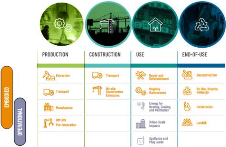
Figure 3: Differences between embodied and operational emissions for a building’s lifecycle (Source: Programme and Architecture 2023)
