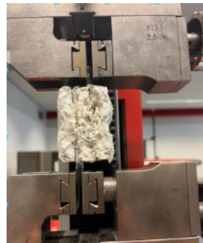
Figure 3: Lap shear test machine with a clamped sample
