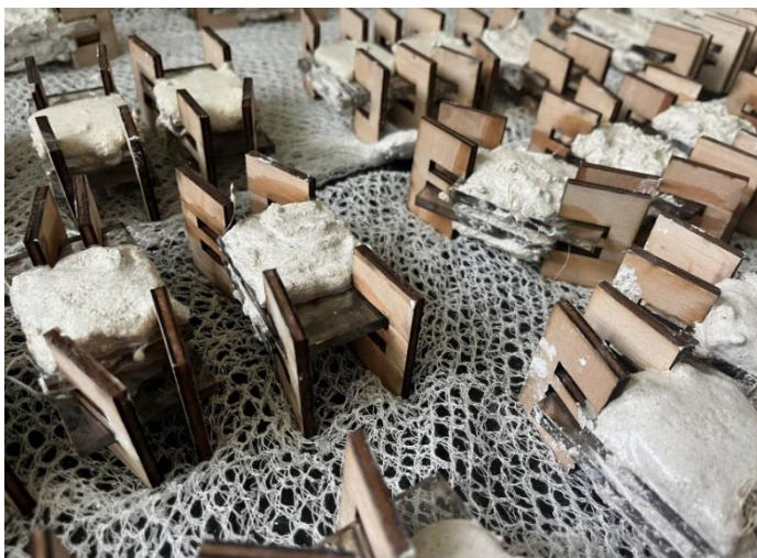
Figure 2: Samples designed for testing shear resistance of assembly
