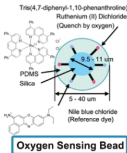
Figure 9: The oxygen sensing microbead fabricated by Wang et al. Containing a silicon core and PDMS shell. The oxygen sensing dye used was Ruthenium(II)Dichloride and the reference dye was Nile blue chloride. Figure from: [60]
