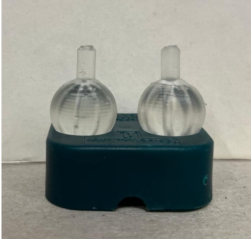
Figure 10: Channel phantoms, one with eight 1.1 mm diameter channels (left) and one with eight 2.2 mm diameter channels (right). Both have a 1.1 mm diameter channels straight through the middle.
