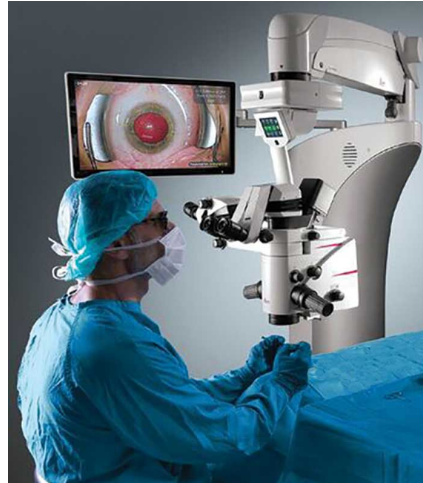
Figure 6: A surgeon looks through the eyepiece of an surgical microscope at the surgical area, which is also visible on the monitor. [35]
