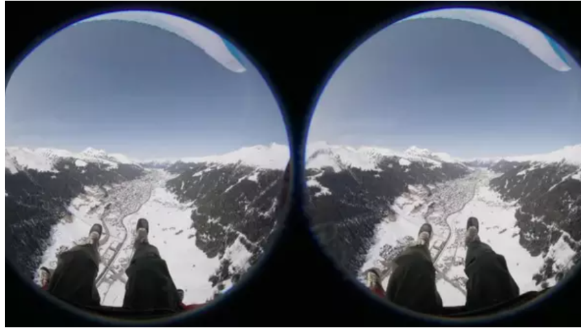
Figure 8: Image showing a stereoscopic view in a VR headset, where two slightly different images are projected to each eye to create a 3D image. [38]
