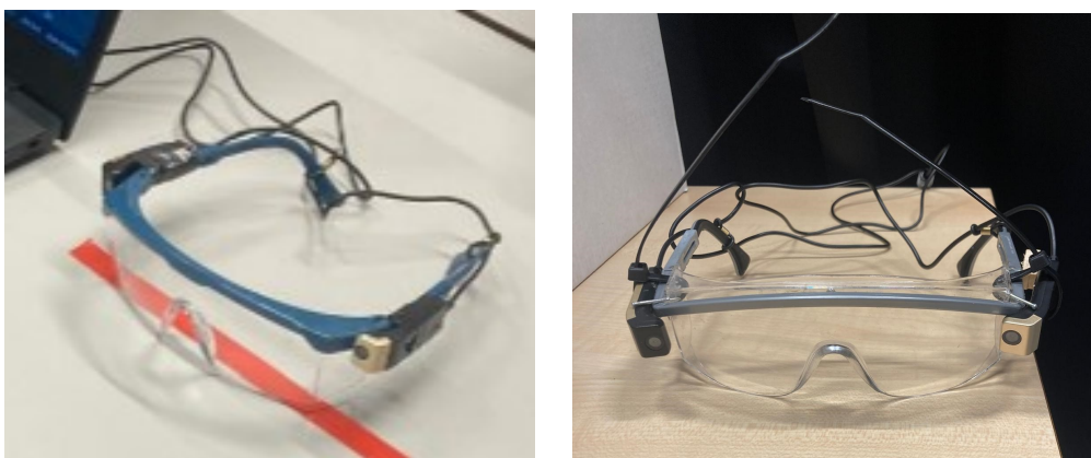
(a) Early prototype of camera-equipped glasses. The cameras are attached to the temples using the camera clips and insulating tape over them.
