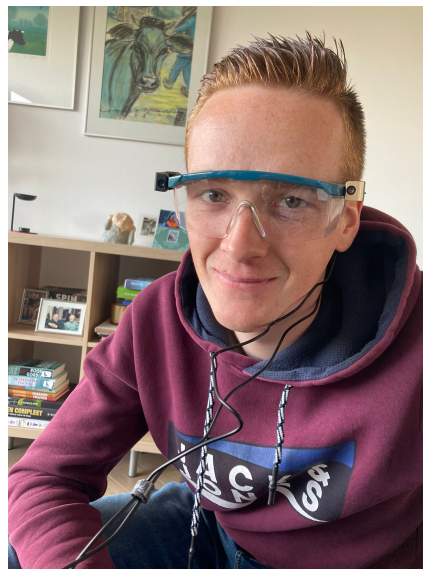
Figure 7: A person wears camera-equipped glasses connected to a laptop via wires. The cameras are attached to the temples of the glasses with clips, and additional stability is provided with insulation tape.
