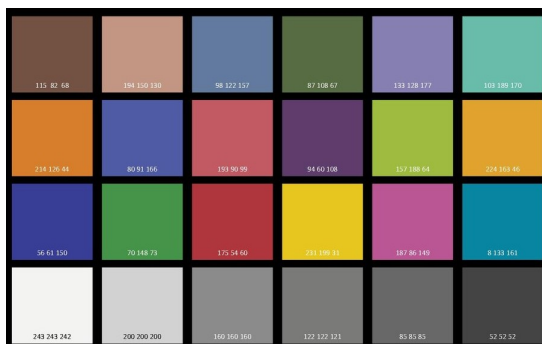
Figure 15: MacBeth ColorChecker used for evaluating colour accuracy. [45]
