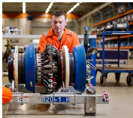
Figure 1 An in-line inspection tool (Company X, 2020)
