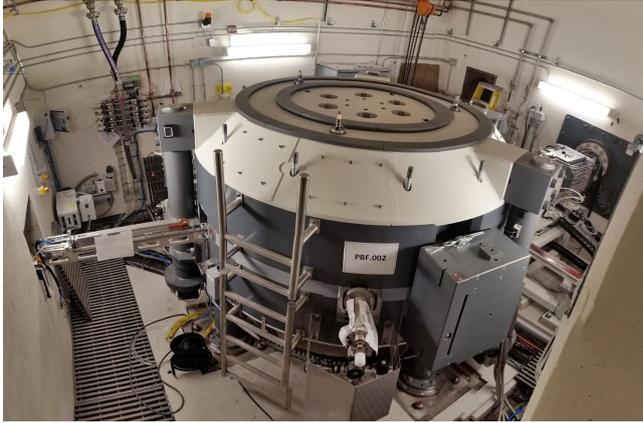
Figure 3: The cyclotron accelerator used in the proton therapy solution, ProteusONE by IBA [15].
