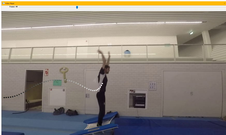
Figure 4.17: Center of mass prototype: calculates and displays the center of mass of the athlete for the current and previous frames
