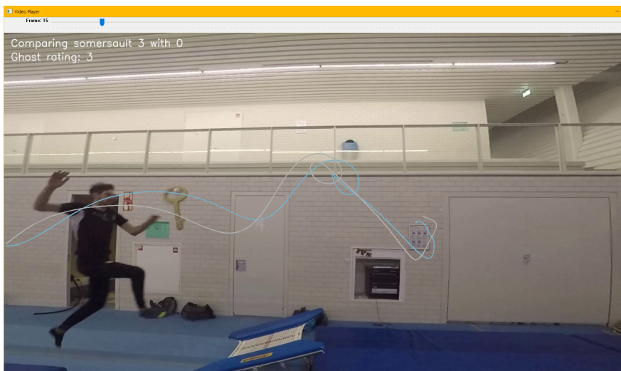
Figure 4.16: Body part tracking prototype: shows the trajectory of a body part (in this case: right shoulder) of the current somersault and a rated comparison
