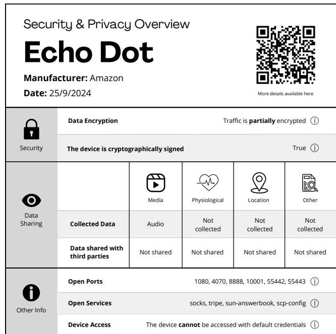
Fig. 12. Automatically generated label for the Amazon Echo Dot. The label provides an overview of the device’s security and privacy features extracted using SPIoT . The label also features a QR code for users to access more detailed information from the manufacturer’s webpage.
