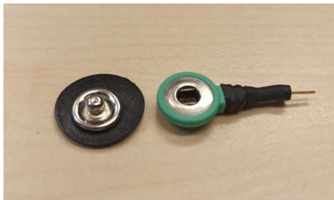
Figure 4.3: An electrode with a snap button attached (left) and the corresponding connector (right).
