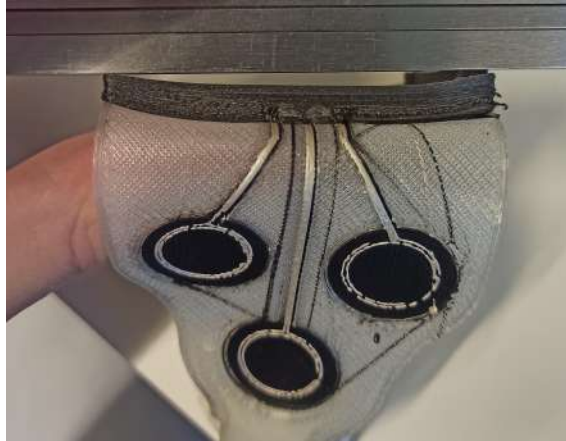
Figure 4.5: An example of the electronics box warping.
