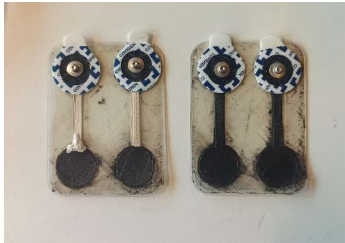
Figure 4.2: One electrode pair connected with silverink (left), one with PI-ETPU (right). Both use sEMG stickers.
