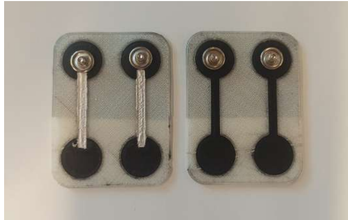
Figure 4.4: One electrode pair connected with silverink (left), one with PI-ETPU (right). Both use metal snap buttons.
