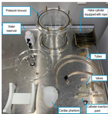
(a) Materials needed to achieve the set up visible in b).
