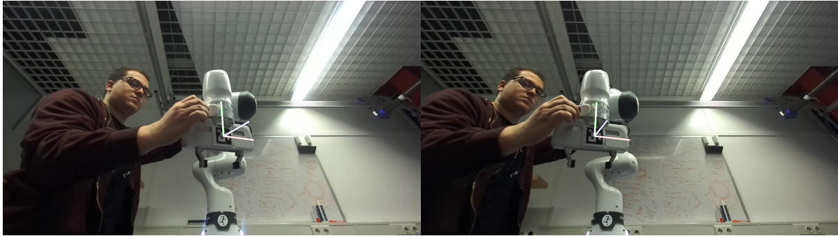
Figure 3: Here an ArUco marker attached to the end-effector is shown that has been processed, the computer recognized the 3 Cartesian's directions stemming from the marker.
