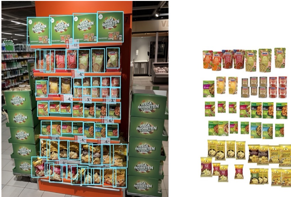
FIGURE 20: Product recognition output for an image from the internal dataset. On the left: the input image with detected products marked by bounding boxes. On the right: the recognized products displayed at the corresponding locations in the input image. Segmentation masks have been omitted for the sake of clarity.
