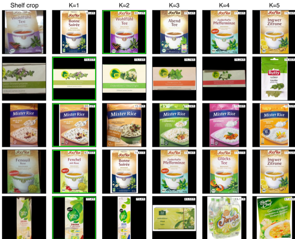
FIGURE 19: Predictions of the classification model for products from the GP dataset. The leftmost column depicts products cropped from the shelf, while the columns to the right show the predicted top-5 most similar packshots. The numbers represent the similarity scores between shelf crops and packshots.
