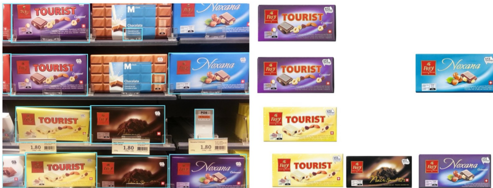
FIGURE 21: Product recognition output for an image from the GP dataset. On the left: the input image with detected products marked by bounding boxes. On the right: the recognized products displayed at the corresponding locations in the input image. Segmentation masks have been omitted for the sake of clarity.
