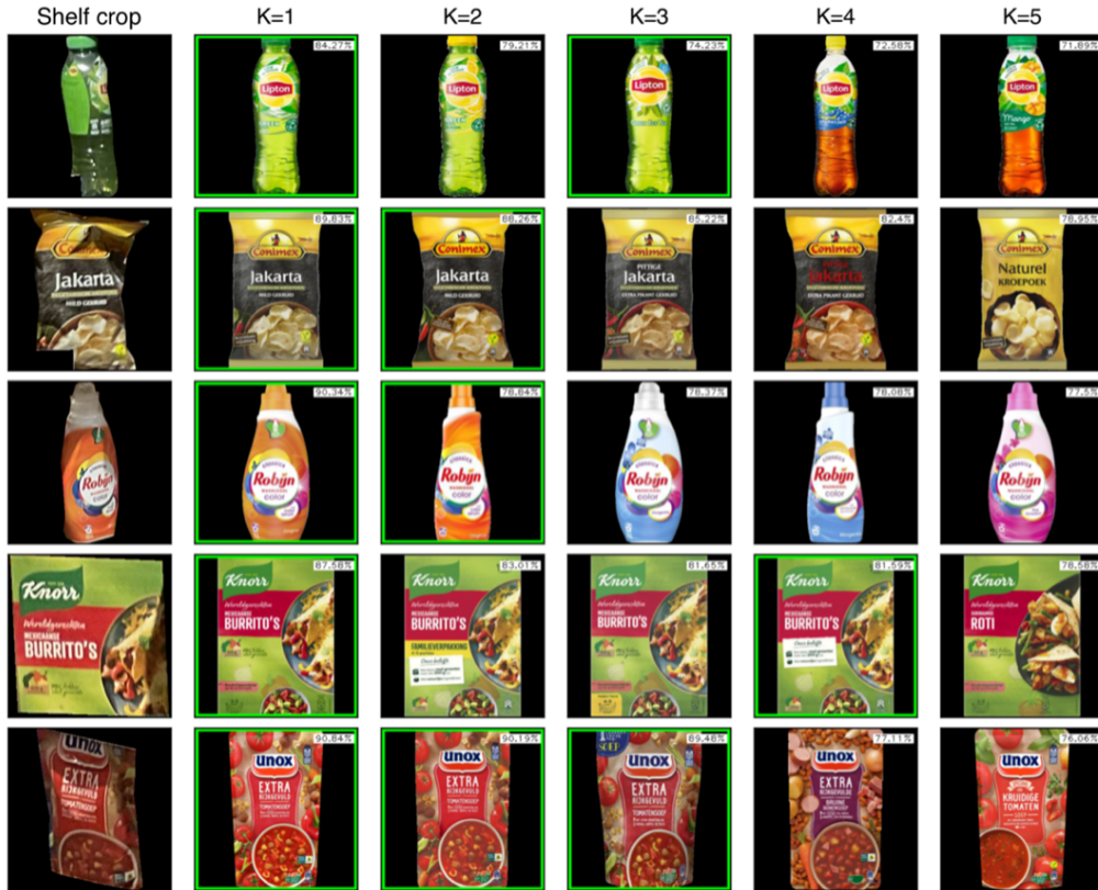
FIGURE 18: Predictions of the classification model for products from the internal dataset. The leftmost column depicts products cropped from the shelf, while the columns to the right show the predicted top-5 most similar packshots. The numbers represent the similarity scores between shelf crops and packshots.
