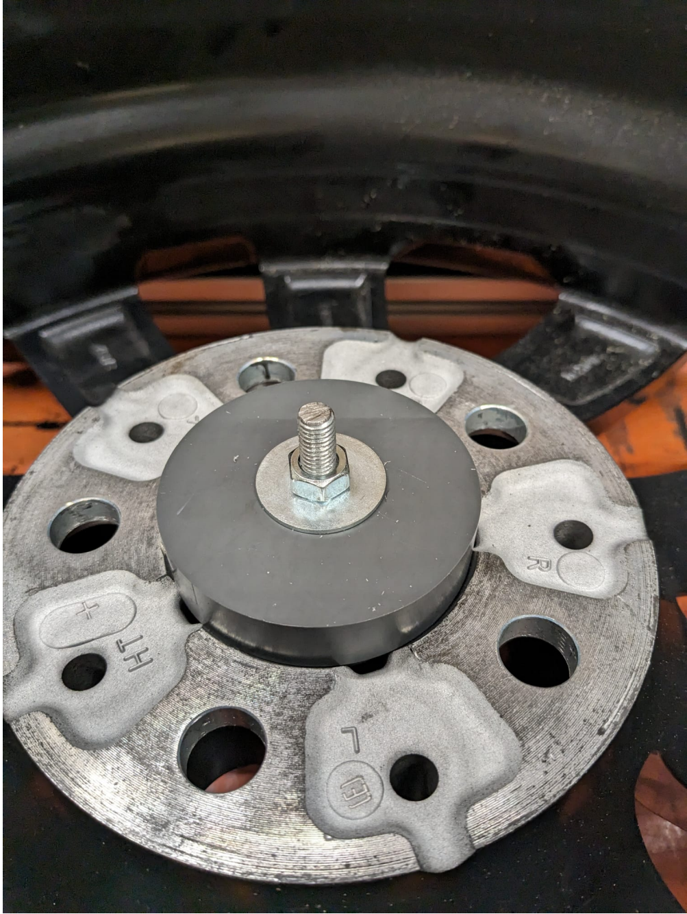
Figure A.3: Mechanism to keep tire positioned in middle
