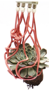
(b) A gripper inspired on the anatomy of a jellyfish [5]
