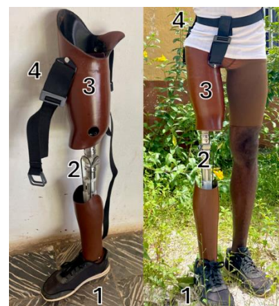
Figure 1: Transfemoral prosthesis, consisting of a foot (1), knee (2), socket (3), and suspension system (4).
