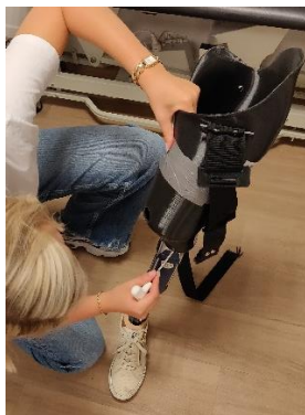
Figure 21A: preparation of the prosthesis, by replacing the socket with the 3D printed socket, and attachment of the silesian belt.
