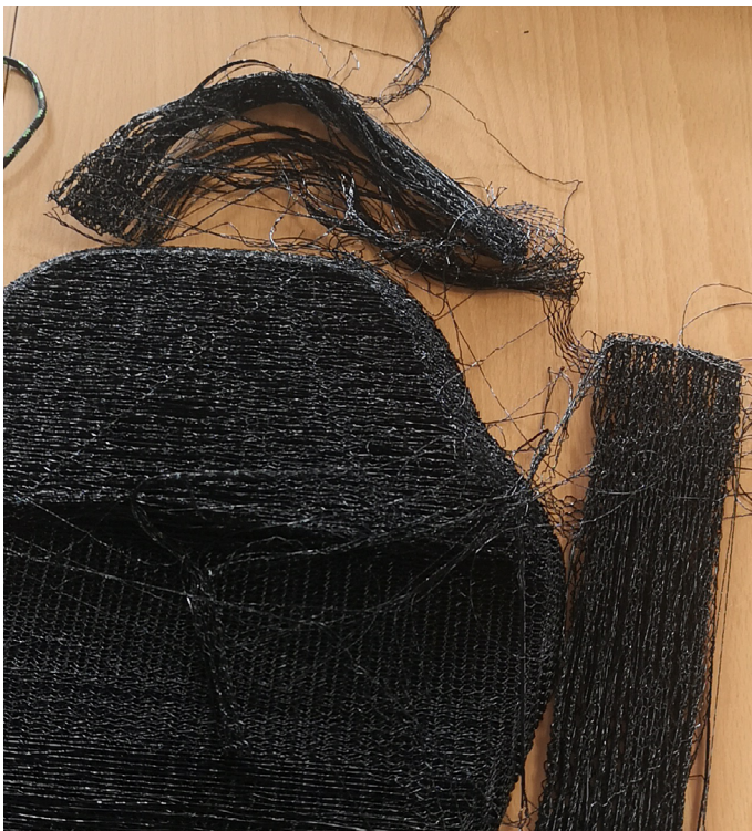
Figure 32: Failed print of the TPU architected back protector insert Own work
