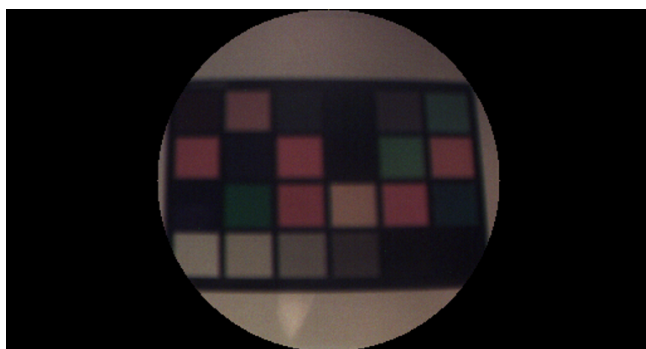
(a) Image created with the RGB-page of the color checker in (b) with wavelengths: 618nm (R), 563nm (G) and 500nm (B)
