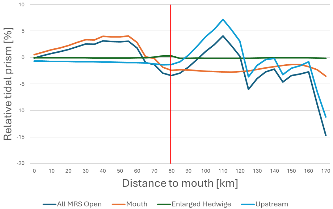
Figure 7 Relative effect of the tidal prism, in red the location of the Hedwige MRS.
