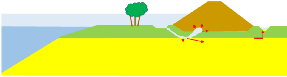
Figure 7: How a burrow can shorten the seepage length, increasing the risk of piping (Deltares, 2023a).
