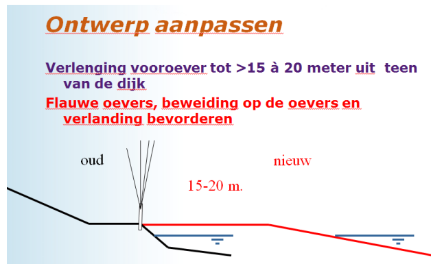
Figure 9: Extending the foreshore as a mitigative measure against animal burrows (Waterschap Rivierenland, 2016).
