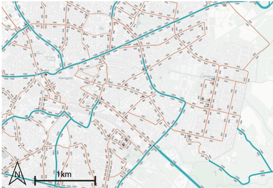
Figure 5.8 Road capacities in Hengelo (Source: OmniTRANS).
