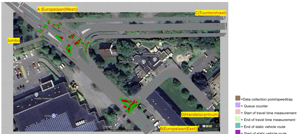
Figure 5.1: Current infrastructure situation model in Vissim
