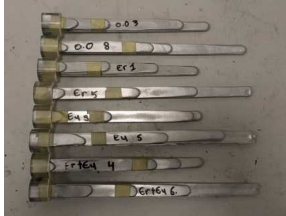
Figure 4.7: Arms of the shortest and longest fluidity casting per composition were embedded for microstructural analysis
