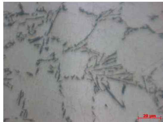
(b) A356 microstructure with plate-like Si [8]
