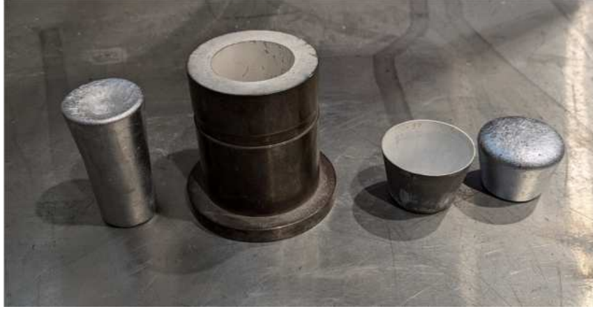
Figure 4.1: Left) Barker sample solidified in copper mold. Right) RPT sample solidified under partial vacuum (80mbar) in thin steel mold
