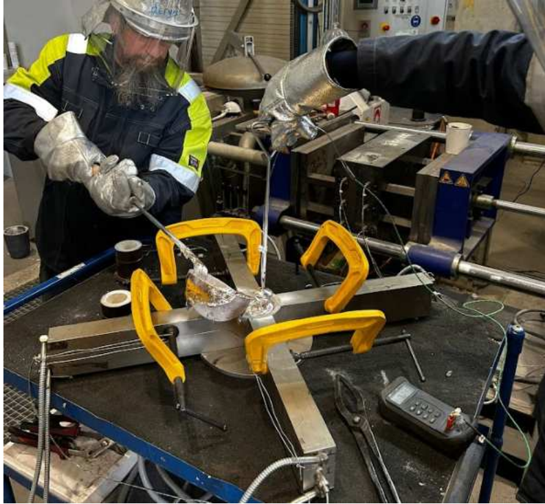
Figure 4.2: Radial Quad setup during fluidity test
