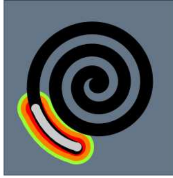
Figure 3.1: Preheating later sections of channel by introduction of melt to the mold
