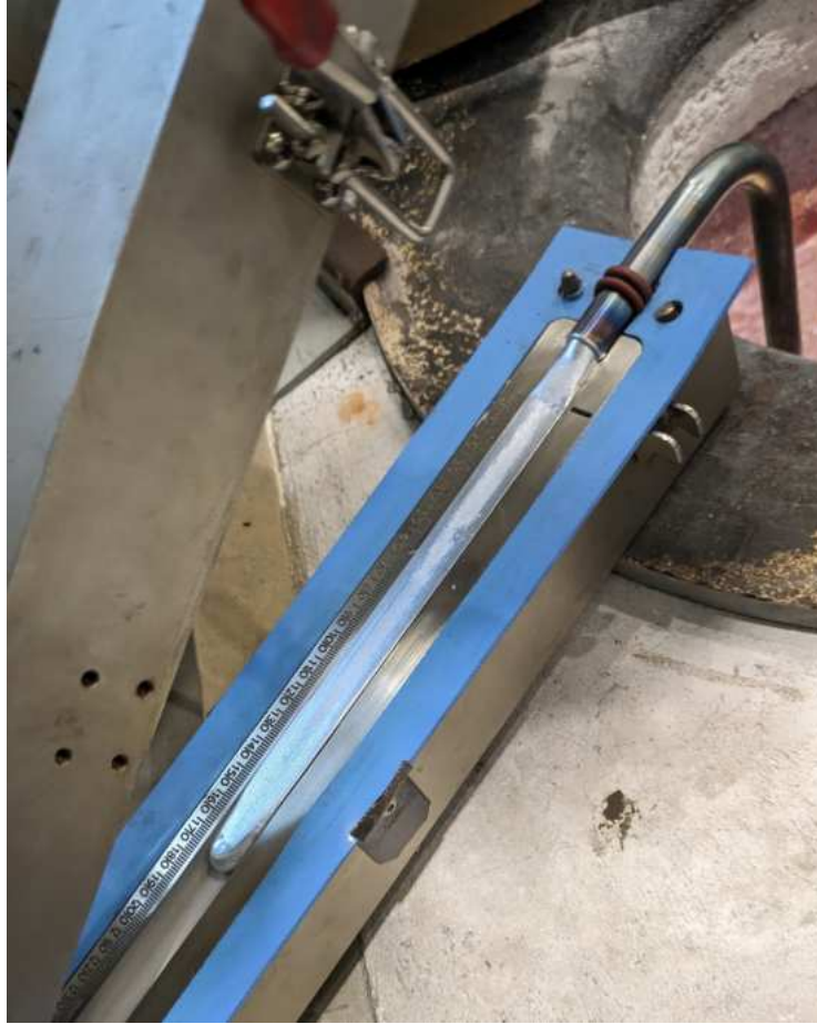
Figure 4.3: Vacuum setup opened after fluidity test
