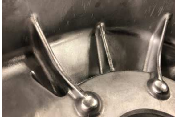
Figure 2.23: Structural ribs in casting, where the thickness to height ratio is small [65]
