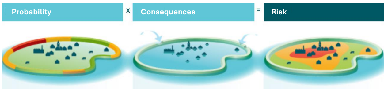
Figure 11: Schematic representation of flood risk calculation (Eems et al., 2018)
