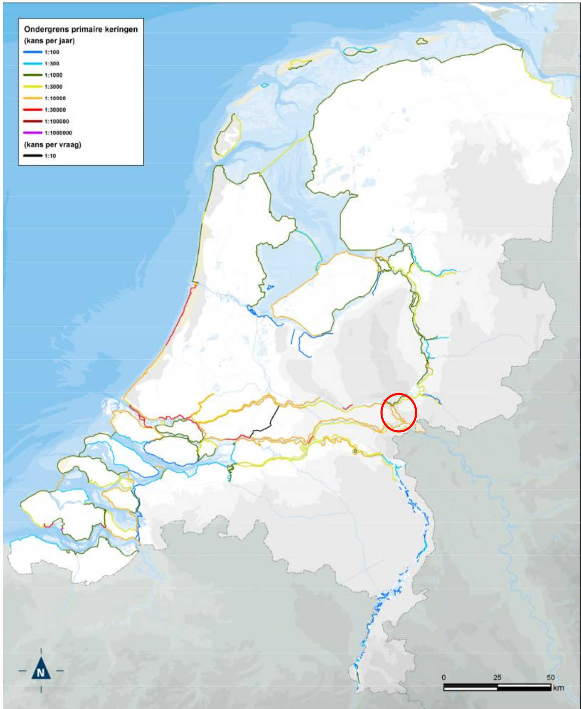
Figure 2: Minimum safety standards for all dike sections. A red circle is added to highlight the case study area (Ministerie van Infrastructuur en Milieu & Rijkswaterstaat, n.d.)
