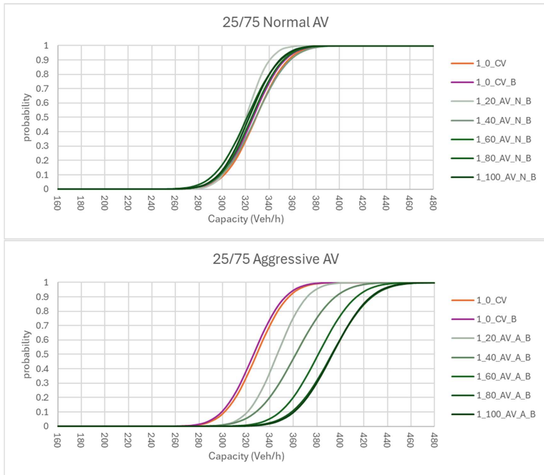
Figure 16: Entry capacity CDF Graphs of different Vehicle Types for Traffic Scenario 25/75 with cyclists.
