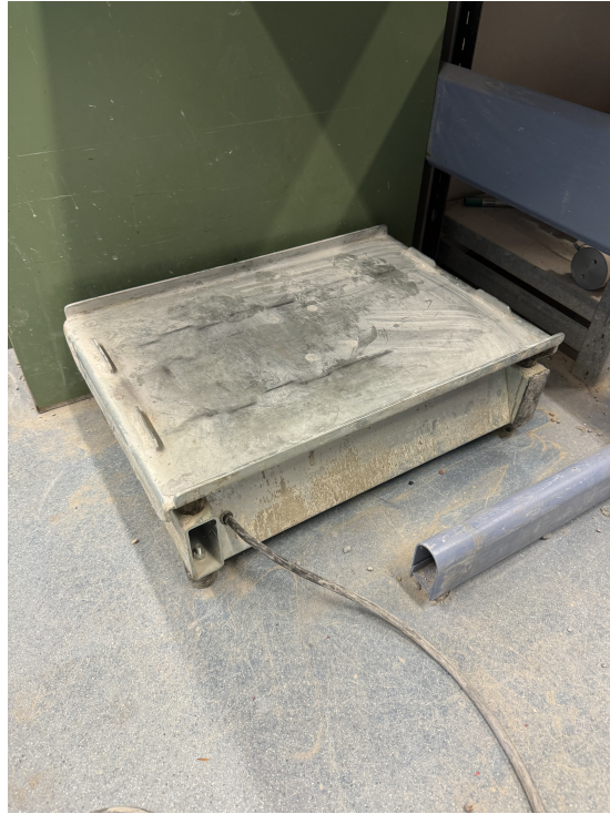
Figure 8: Shaking machine used to carry out the void ratio experiment
