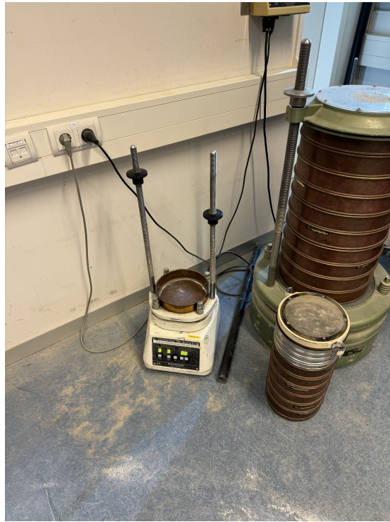
Figure 9: The sieving equipment used to conduct the Particle Size Distribution
