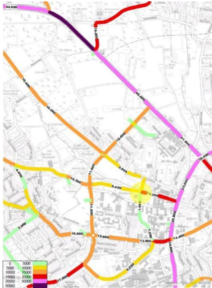
Figure 2.6: Traffic prognosis considering MMQ1 and MMQ2 developments, with the intersection marked in yellow. Adapted from [2].
