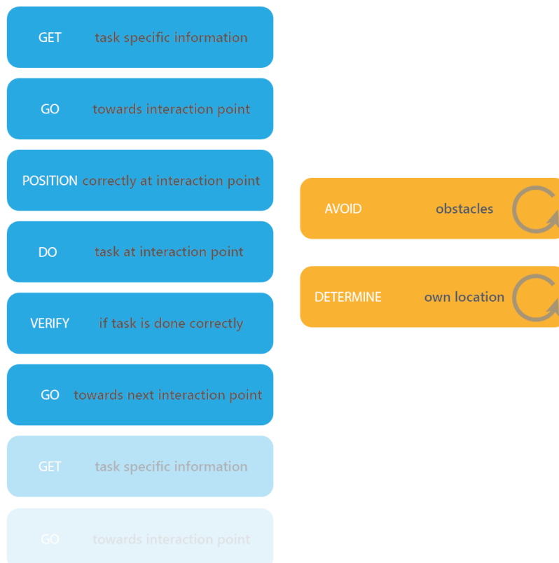
Figure 6: Overview of the generalized functions of a turnaround task. The left shows the consecutive steps, the right shows the continuous steps
