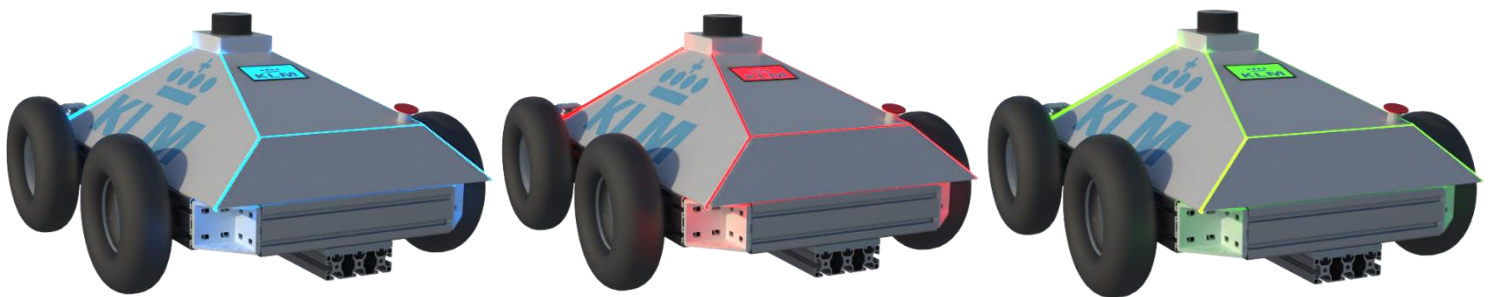
Figure 27: Renders of the WCR displaying different phase light colours. Blue, red and green from left to right
