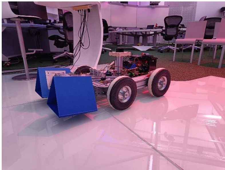
Figure 38: Picture of the prototype that is carrying the mock-up wheel chocks
