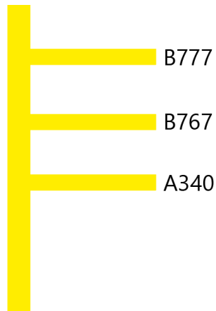
Figure 8: Illustration of the centreline markings for the aircraft on the aircraft stand
