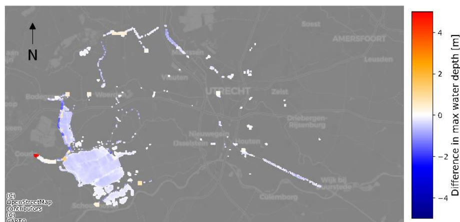
Figure 18 - Difference in water depth on the 2D grid between the benchmark and SUG #D2 (resolution of 500 m). Blue indicates that the water depth in the surrogate is smaller than in the benchmark model.
