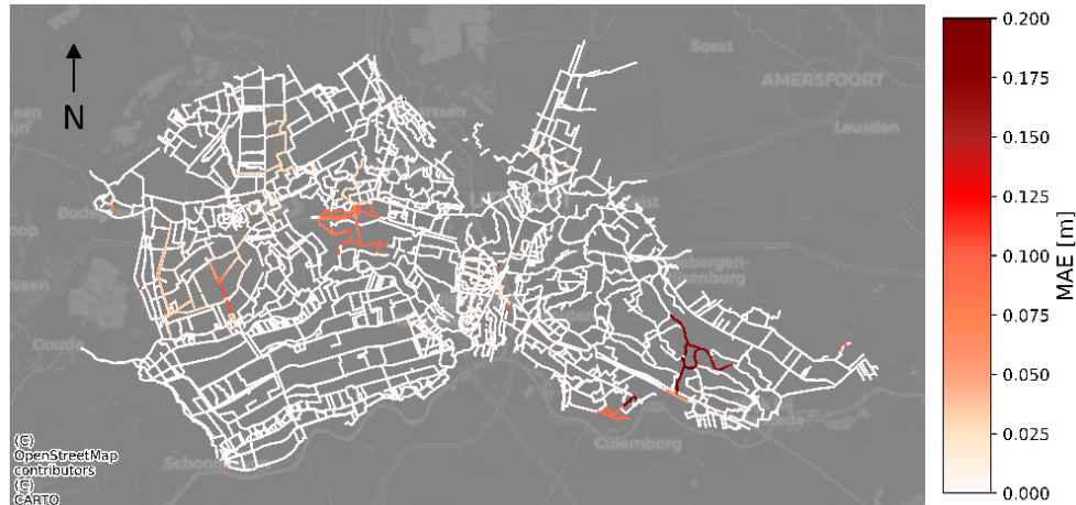
Figure 13 - MAE of the maximum water level in the 1D network for SUG #C2.
