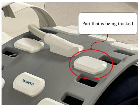
Fig. 6: The MRI receiver coil of which the movement is being tracked to capture the subject's external motion that is caused by breathing.
