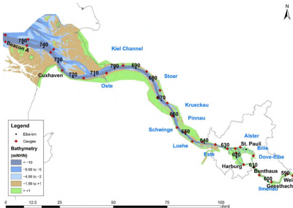
Figure 2.2: Map of the Elbe estuary, with colours indicating the bed levels compared to the mNHN (German Normalhöhennul, which is equal to NAP), numbers refer to Elbe-km (S. Hein et al., 2021)
