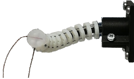
Figure 13: Close-up on the endoscope with the 6-DOF EM tracker connected. The two wires running out the cap on the endoscope are from the two 5-DOF EM probes.
