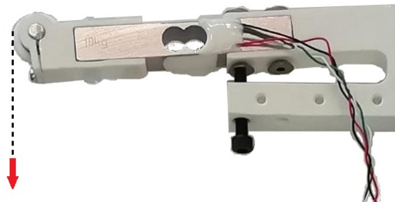
Figure 7: Tension sensing unit. The load cell (in the middle) is encased by 3D printed parts on both sides to fixate it and guide the wire along the sensor. Forces along the dotted line marked with the red arrow are measured.
